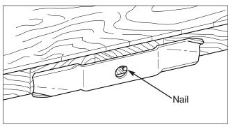
Figure 26. Balancing The Blade
